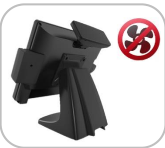
Aluminum die-casting chassis fanless design
